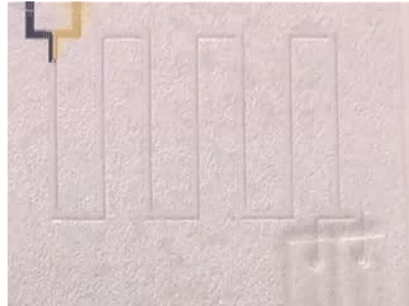
demonstration of laminar flow (Nanostream; USA)
