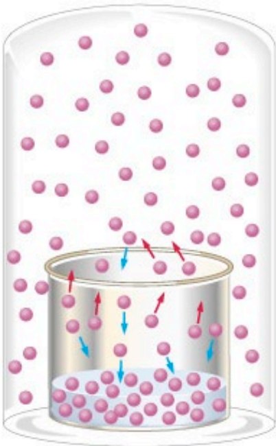
(c) Vaporization rate = condensation rate
