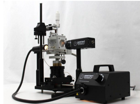
Fig. A.1. Droplet-volume method to determine interfacial surface tensions
