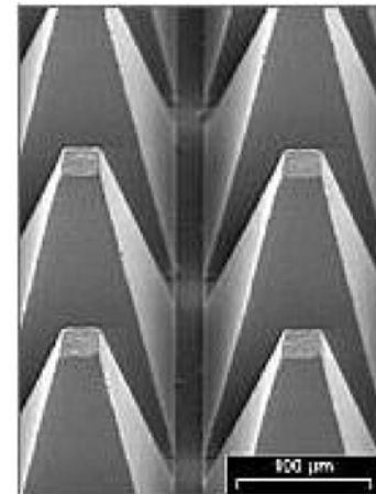
Fig. 4.21. Mold master fabricated by mechanical machining
