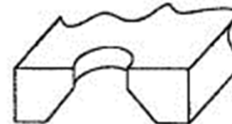
Tapered with cylindrical exit orifice (Seiko-Epson)
