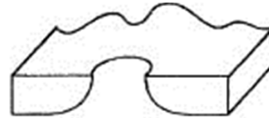
Convergent orifice (HP, Dataproducts)
