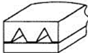
Triangle orifice (Xerox)
